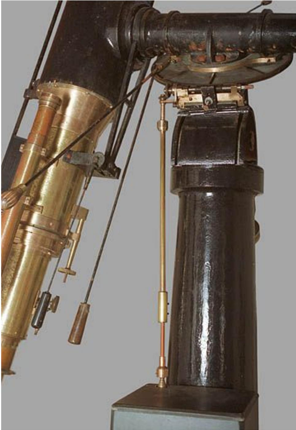
**Fig. 4.** Close-up of the equatorial drive system and coupling rod
