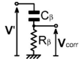
If we now choose  $C_\beta$  to be the same as  $C_\alpha$ , then setting  $R_\beta = R_i / N_i$  gives the required correction voltage, except that the sign should be negative (phase reversal is required).
