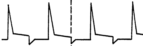
Fig. 4 TRANSISTOR BASE CURRENT
