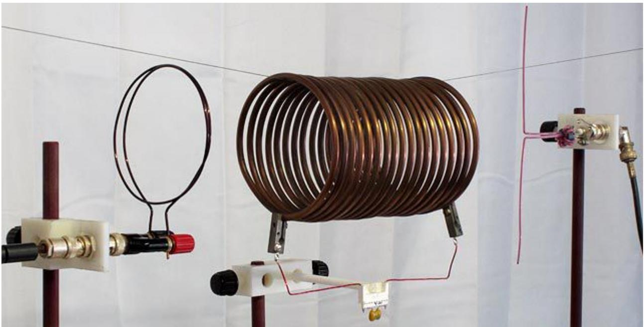
**Variant of the Howe extrapolation method for self-capacitance.** By connecting only the reference capacitor to the coil, the lead correction is greatly simplified. The RF source connected to the induction loop (upper photograph) is an MFJ269 impedance analyser; floated from ground (in addition to the unun in the antenna cable) by placing a ferrite isolator in the power cable, and by attaching the tuning capacitor to a long non-conductive extension spindle and reduction drive.
