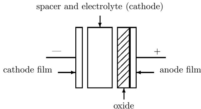
Figure 6: Cross Section of Aluminum Electrolytic Capacitor
