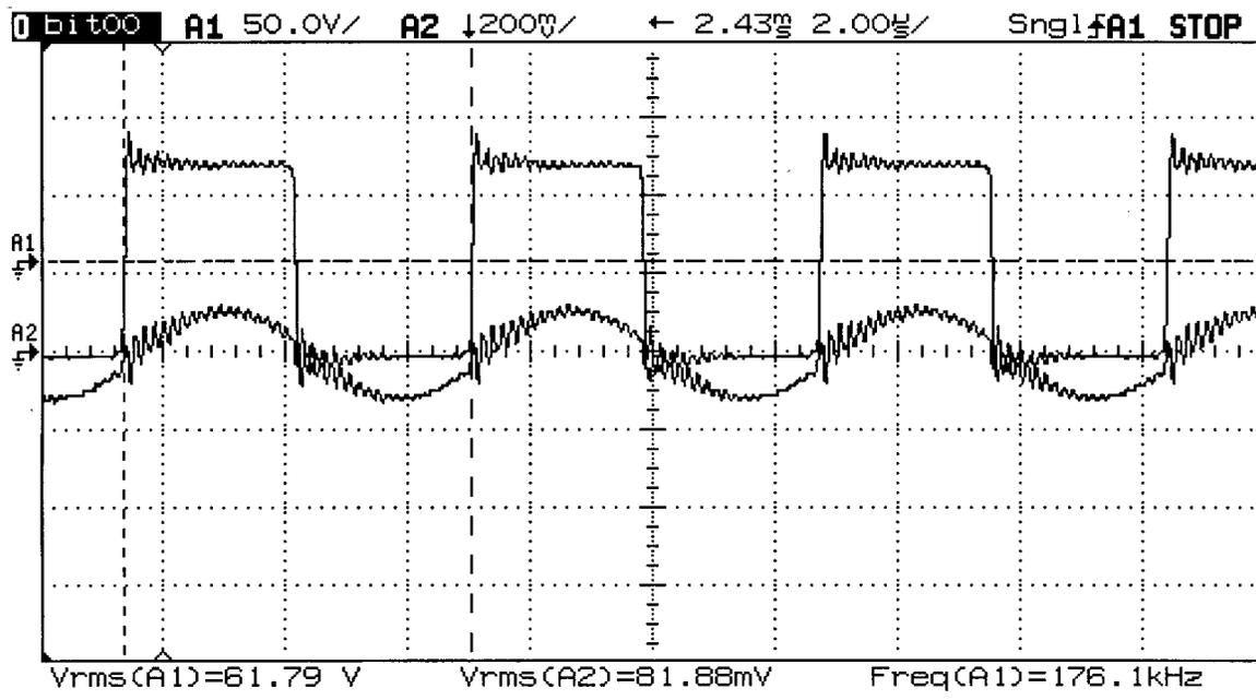
Figure 4: Voltage and current during spark at variac = 40%
