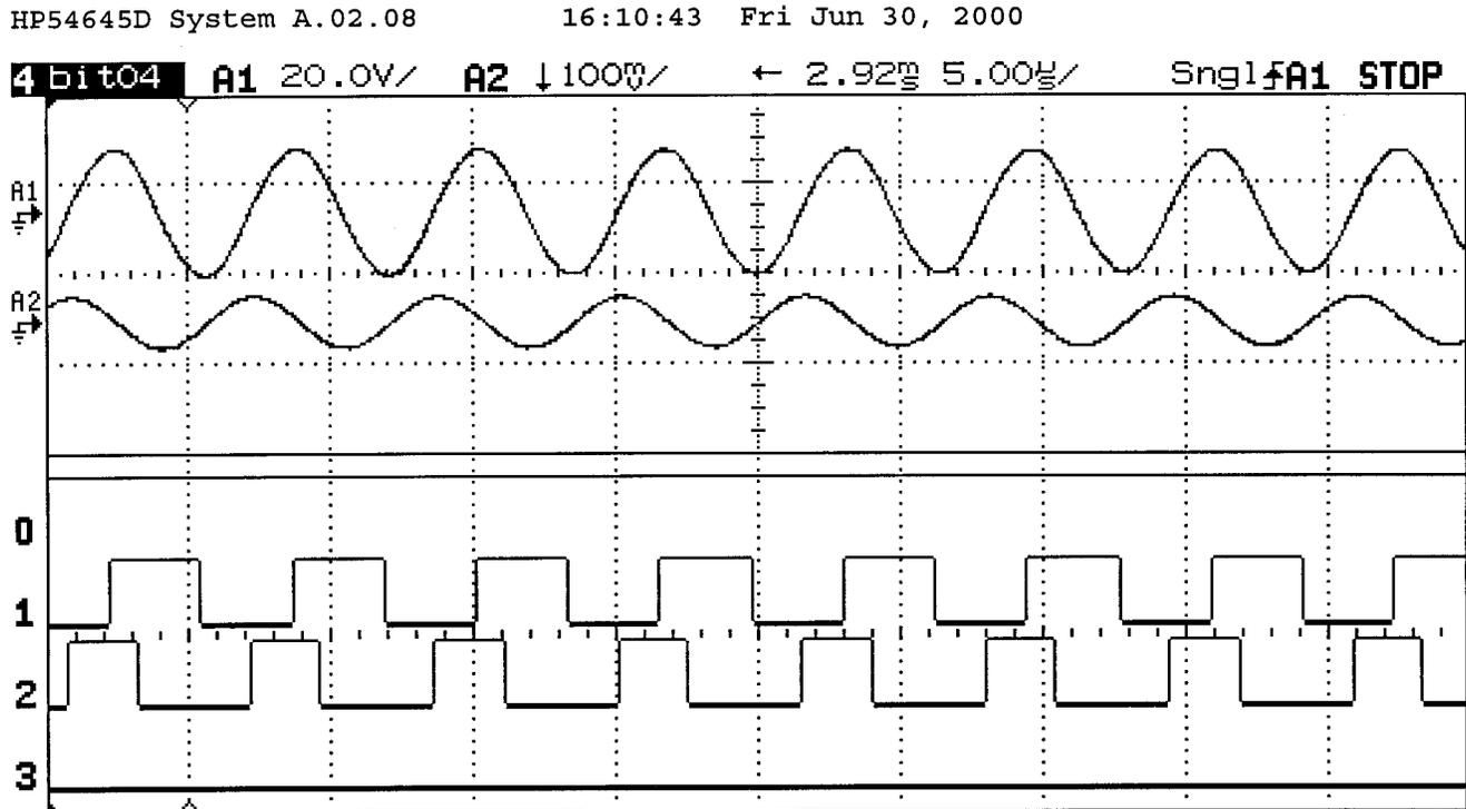
Figure 11: Voltage and Current During Ring Down
