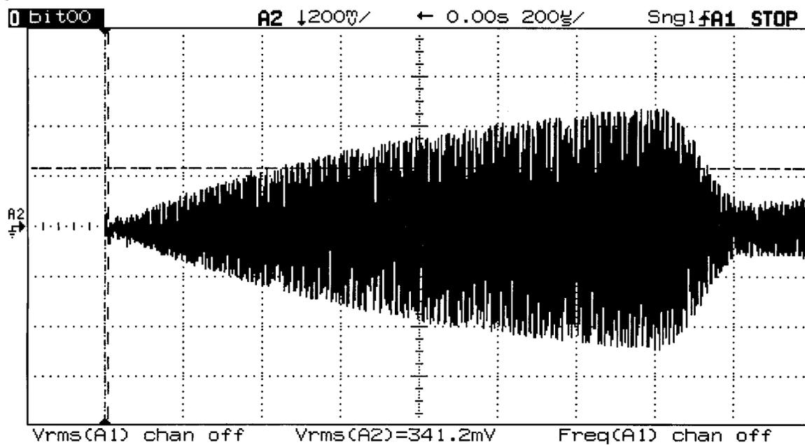
Figure 2: Current waveform at variac = 40%
