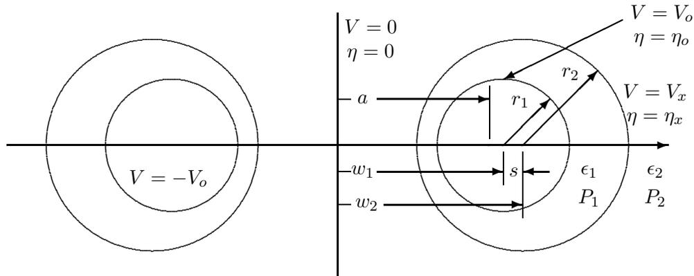
Figure 5: Two Adjacent Turns of Magnet Wire
