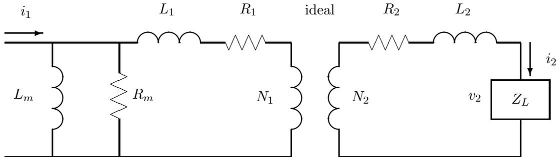
Figure 8: Transformer Model
