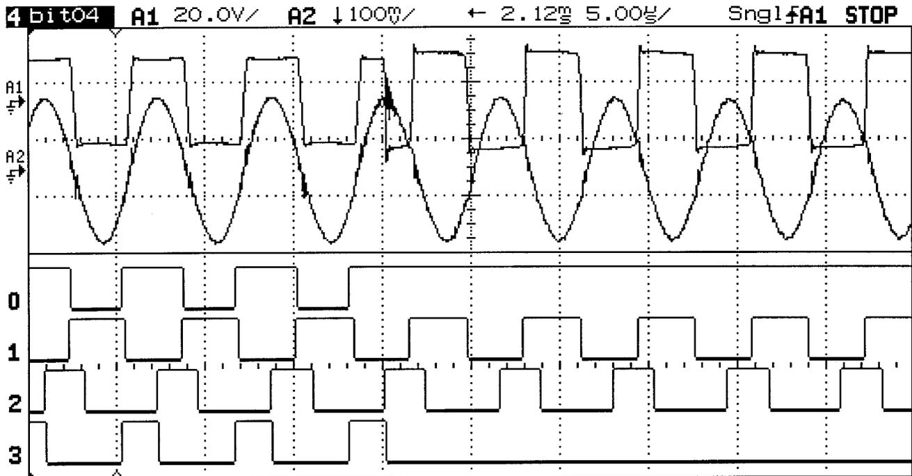
Figure 10: Voltage Phase Shift at ENABLE Turnoff
