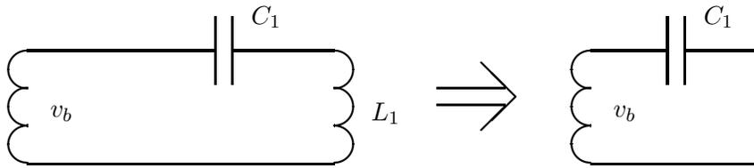
Figure 2:  $C_1$  Being Charged With The Gap Open
