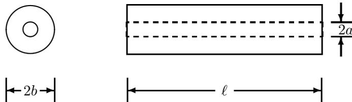
Figure 5: Coaxial Cable
